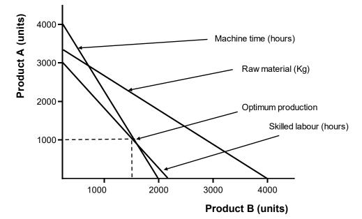
Graph showing constraints and optimum production plan
